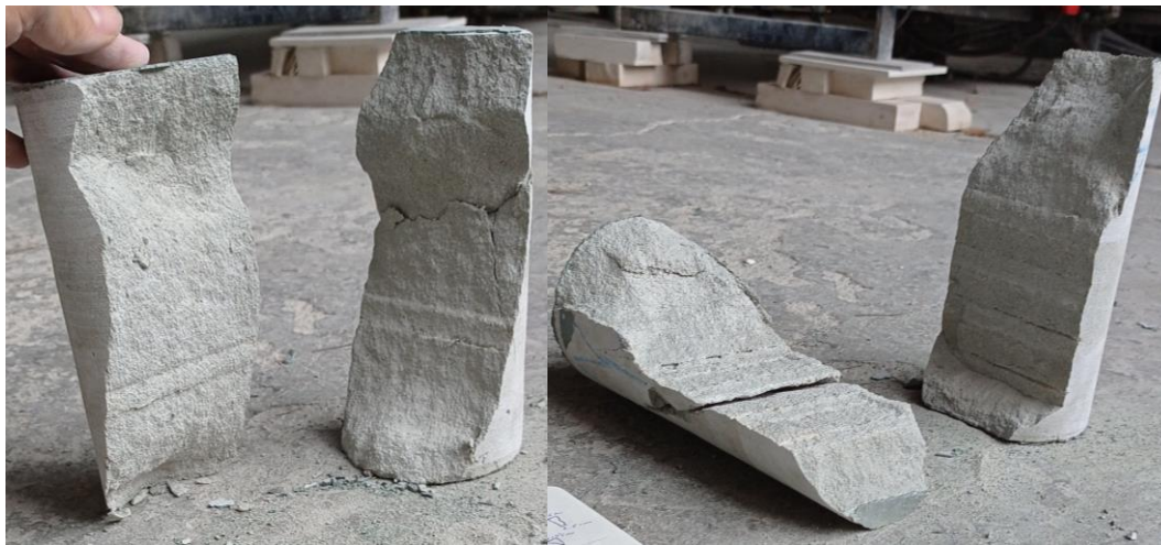
(a) Failure mode of U_{Y-S2} and U_{Y-S5} , respectively
