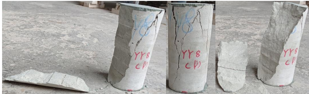
(a) Failure mode of U_{Y-D8}
