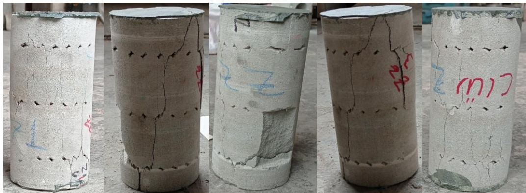
(a) Failure Modes of U_{Z1} , U_{Z3} (Front View), U_{Z3} (Right Face), U_{Z3} (Left Face), U_{Z9} , respectively.
